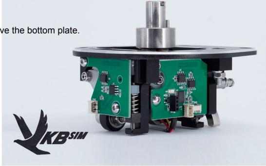
\*Note: The inner 4 screws are fixed in place with locktite and are not meant to be removed by the user!
